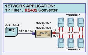
Fiber 485/232<sup>®</sup> Models 4149 & 4159 Very High Speed Ruggedized Fiber to RS485/422/232 Interface Converters
