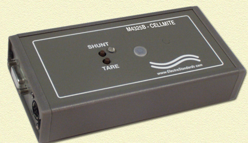
Model 4325B CellMite® Intelligent Digital Signal Conditioner
