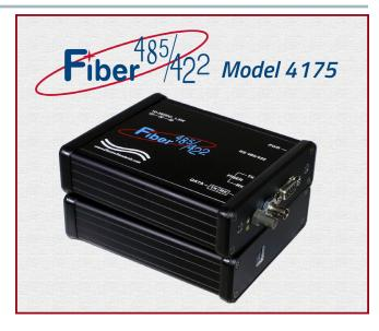
3kVDC isolation to prevent system ground loops. It can be powered from a wide input range of 10VDC-36VDC, with models also available for other voltage ranges such as 4.5VDC-9VDC and 19VDC-72VDC. Other features include user selectable fiber polarity, and also TX, RX and Power indicator LEDs.
