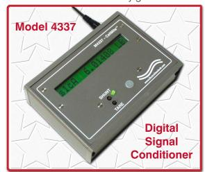
The CellMite® Model 4337 can be fully operated with a computer or simply setup by a computer and then used as a stand-alone intelligent digital signal conditioner with auto identifying analog and alphanumeric display outputs.
