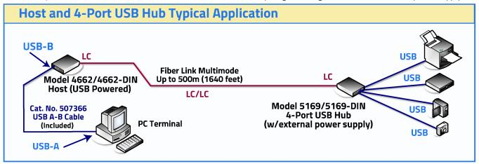
USB A-B Cable (6 FT): Included with Model 4662 / 4662-DIN is the cable ESL Cat. No. 507366. (USB Type A to USB Type B)
